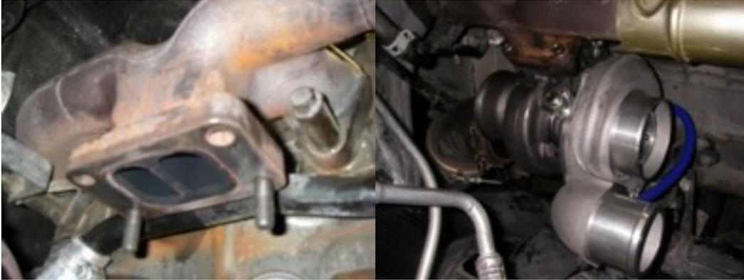
**Step 11:** Reinstall exhaust, intercooler pipe and oil feed line. Leave the turbo side of the oil feed line a couple turns loose until the final step. You may have to bend the dip-stick tube slightly to make room for the new down pipe position on trucks with automatic transmissions.
