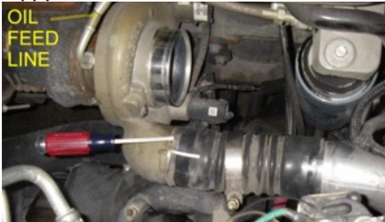
**Step 4:** Remove top exhaust clamp from exhaust elbow and loosen the bottom one so the elbow spins freely. Next, unclip boost sensor from turbo. Then, from under the truck, notice how far the oil drain tube on the turbo is seated into the block. Push up on this tube and it will pop out of the block, being careful not to kink this line.
