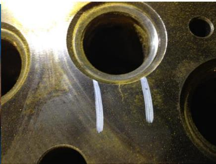
Cracks in head or block
